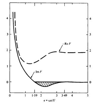
FIGURE 2. Variation of the real and imaginary parts of  $F(\epsilon)$  defined in (2.29) as a function of the reduced frequency  $\epsilon = \omega s/U$ .
