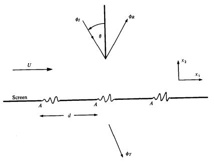
FIGURE 3. Diffraction of sound by a perforated screen in the presence of a uniform mean flow in  $x_2 > 0$ .
