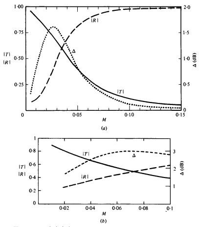
FIGURE 4. Variation of |T|, |R| and  $\Delta$  (a) with the mean-flow Mach number M in  $x_2 > 0$ , (b) with the mean flow on both sides of the screen (after Howe 1980a). The sound is incident normally on the screen, and kd = 0.2,  $\sigma = 0.05$ .
