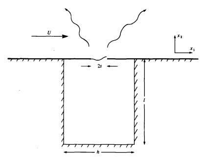
FIGURE 7. The wall cavity. The cavity and the slit have the same length d in the direction normal to the plane of the paper.
