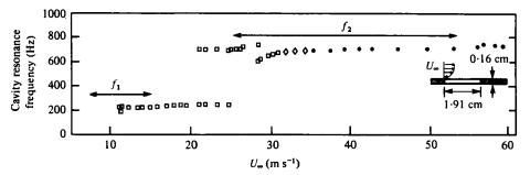
FIGURE 8. Dependence of the resonance frequency of the DeMetz & Farabee (1977) wall cavity on the mean flow velocity. The solid lines represent the velocity ranges predicted by (4.26) in which the resonance frequencies  $f_1 = 200$  Hz and  $f_2 = 700$  Hz are excited by the flow.  $\Box$ , laminar boundary layer;  $\diamondsuit$ , intermittent transition boundary layer;  $\bigcirc$ , turbulent boundary layer.
