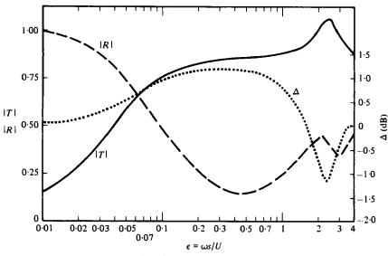
FIGURE 6. Variation of |T|, |R|,  $\Delta$  with the reduced frequency  $\epsilon$  for normal incidence and M = 0.015,  $\sigma = 0.05$ .
